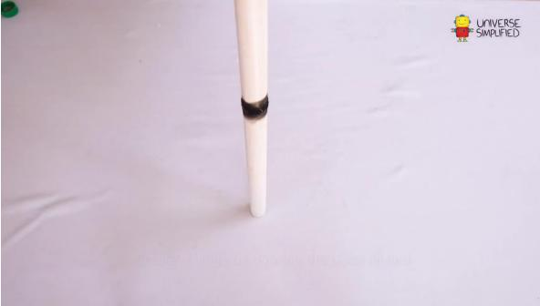
**Step 11**Insert the pipe in the bottle to check that the bottle cannot move beyond the bulge.
