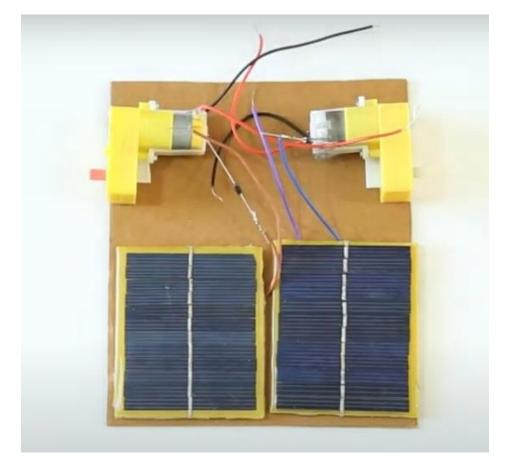
If your cardboard is unable to take the weight of motors and panels, use wooden sticks or metal spokes under the cardboard so that the cardboard has enough support to hold the weight of motors and solar panels.
