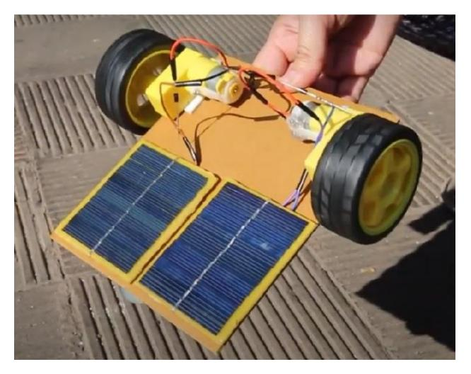
If one of the wheels is moving in the opposite direction, then just reverse the wiring connection of the motor and solar panel (connect Red wire to point B of the motor and Black to A).
